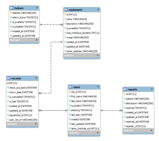
This is the initial database design. The initial design is based off of the use cases we have in mind, and the design of previous groups. After testing, additional fields or tables may be necessary if we find that we want to store more information to allow for additional functionality.
